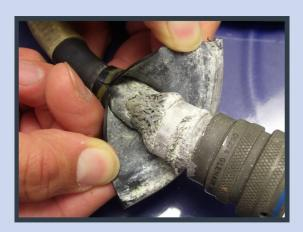
Corrosion can occur when condensation and moisture intrusion get into the back shell of the connector. The majority of aircraft connectors are made of aluminum or steel, and the electrical wire harness endpoints typically consist of wide variety of metals. Adding an electrolyte to the anode and cathode will result in the start of galvanic corrosion.
