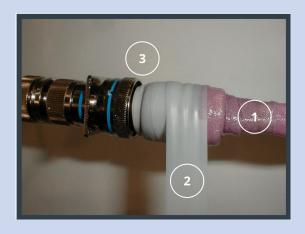
In addition to filling the Connector Backshell with Self-Leveling Green, Av-DEC Dual Wrap Connector Sealing System further enhances protection against moisture and corrosion.
